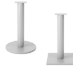
TUBULAR leg WITH BASE PLATE Round 4" diameter tubular leg with round or square base plate. The plate is 18" in diameter or 18" x 18". Height adjustment from 27" to 30" H. Under the surface
